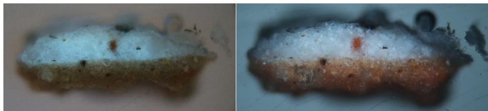
Figure 37: Cross section OL03 in visible light (left) and UV light (right), both at 10x magnification (white spirit)
