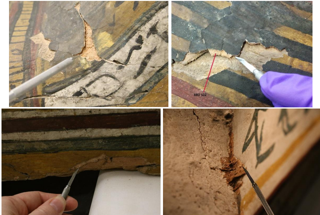
Figure 48: Samples taken from Outer Coffin for XRD analysis: Top row: Outer lid, pink plaster XRD 01 (left); XRD 02 pink plaster from area of historic repair (right); Bottom row: Outer lid, second layer of pink plaster, XRD 03 (left); Outer box, pink plaster XRD 04 (right)
