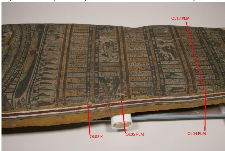
Figure 33: Sample sites for PLM and cross section analysis VI
