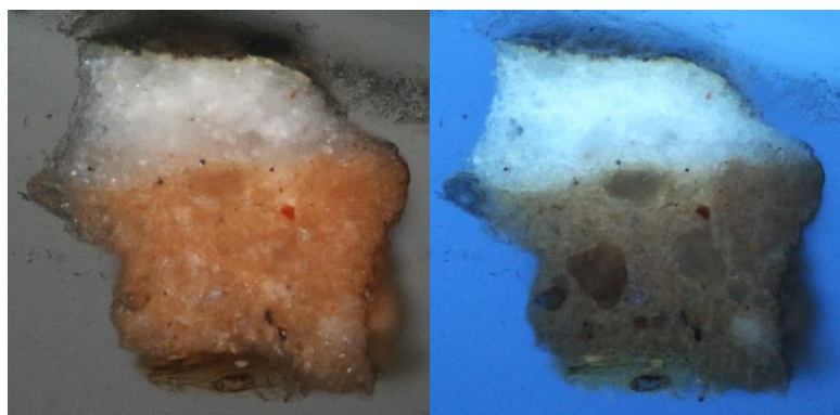
Figure 38: Cross section OL09 in visible light (left) and UV light (right), both at 20x magnification (white spirit)
