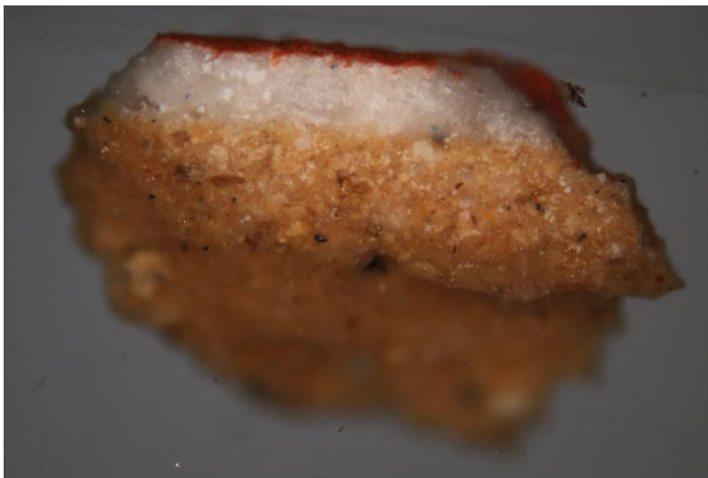
Figure 42: Cross section OB04 in visible light at 5x magnification (white spirit)
