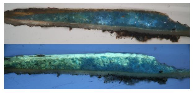
*Figure 5: Cross section IL12, 10x, saturated with white spirit, in visible light (above) and ultraviolet light (below)*
